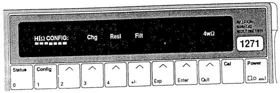
Chg and Resl are menu keys, but  $\underline{Filt}$  and  $\underline{4w\Omega}$  are toggle keys.
