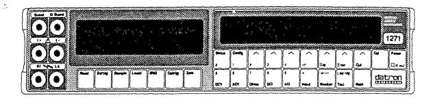
The two displays on the front panel deal with different aspects of operation. We set up the instrument's configuration using menus shown in the right-hand (dot-matrix) display, then readings appear in the left-hand (main) display.
