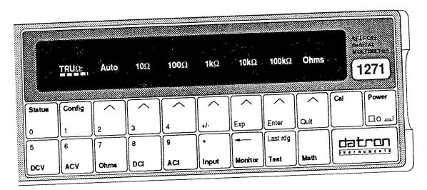
The  $TRU\Omega$  mode generates two readings per measurement. The first is taken with the constant current flowing; the second without the current, measuring any external EMFs that may be present. The difference between the two readings is then calculated, giving an offset-corrected measurement.
