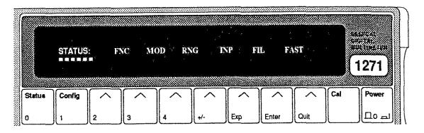
Status is a complete report of the most recent selections made using any of the various menus. It can be used at any time as a fast means of checking that the DMM selections are suitable for the measurement being made.
