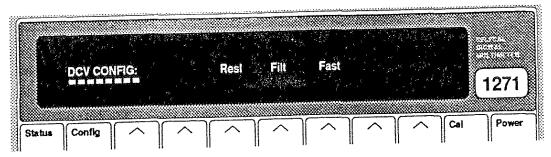
Resl: Displays the DCV RESL menu, to select the resolution for the reading.
