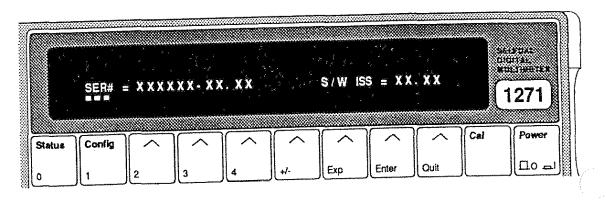
This display is for information only. The serial number cannot be altered except in one of the calibration menus, and this facility is only provided for use during manufacture. Once changed, the number is not lost when the instrument power is turned off. The software issue number (last four digits) is embedded in the software itself, and is not user-alterable.
