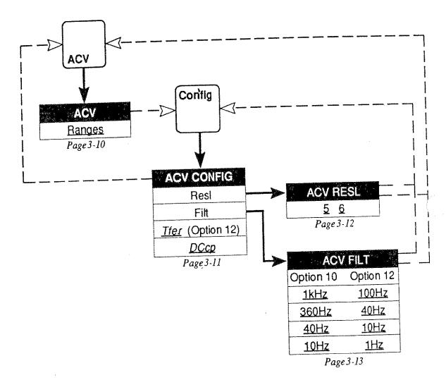
Broken lines indicate use of hard keys
