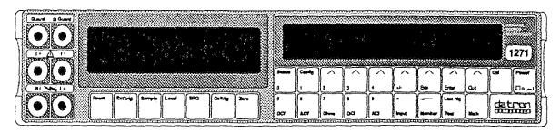
The two displays on the front panel deal with different aspects of operation. We set up the instrument's configuration using menus shown in the right-hand (dot-matrix) display, then readings appear in the left-hand (main) seven-segment display.
