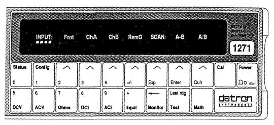
SCAN is a menu which defines only the two keys A-B and A/B. They interact with the other keys of the INPUT menu, so six soft keys are defined. When all six are unselected, an isolated-input state is defined. There is **no** INPUT CONFIG menu.
