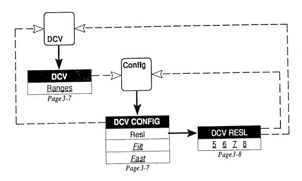
Broken lines indicate use of hard keys
