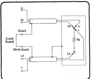
above about  $1M\Omega$ , a metal screen can be wrapped around the resistor to reduce noise. Connecting the  $\Omega$  Guard terminal to the screen will intercept leakage via the screen (in parallel with the unknown resistor). The resistor under test should not be grounded, as this will make the measurement are eliminated. noisier.
