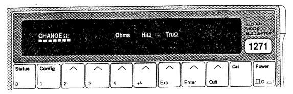
The CHANGE  $\Omega$  menu is accessible from all three Ohms modes, and itself gives access to all three modes. It defines the following menu keys, each selecting a different Ohms mode menu:
